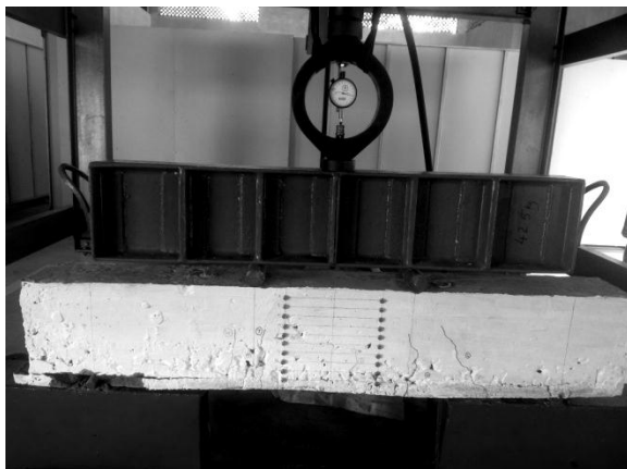
Fig. 4 Failure of Beam Treated with PCM
