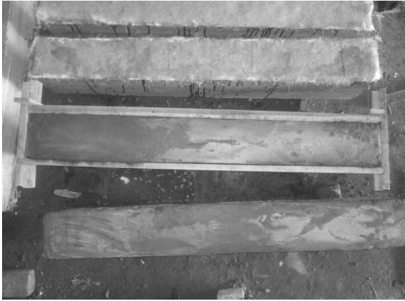
Fig. 2 Beams Treated with GFRP and PCM
